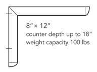
Weight capacity is based on evenly distributed static loads
