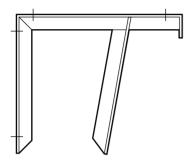
$18" \times 21 \frac{1}{2}"$  counter depth up to 25" weight capacity 450 lbs
