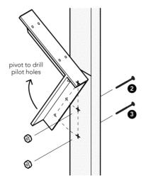
Install the remaining **anchors** and tighten all three until the counter bracket is secure. Carriage bolts should be seated into the wall stud properly.
