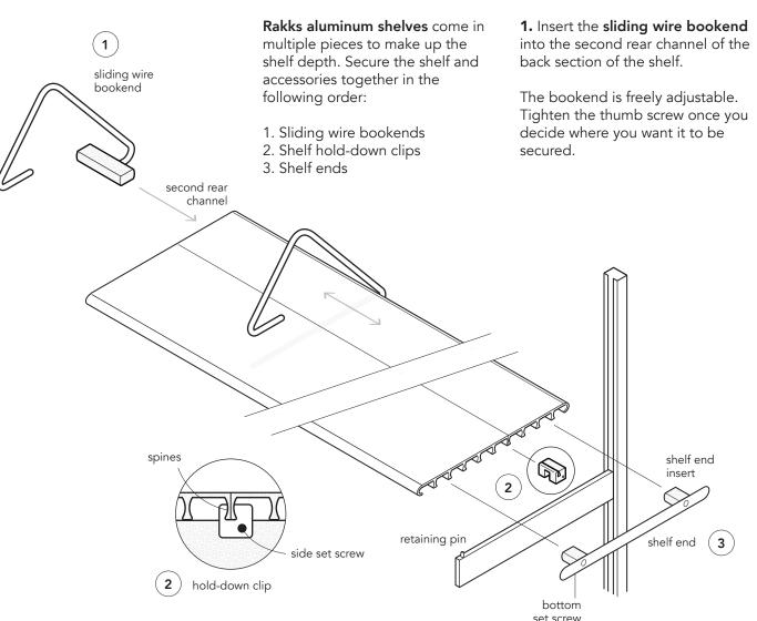
2. Shelf hold-down clips prevent side-to-side movement and hold the shelf firmly in place. They hold together the two adjacent spines of the shelf sections. The notch in the center of the hold-down clip sits over and attaches to the bracket.
