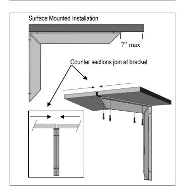
Rakks Counter support brackets come in a variety of sizes, configurations and finishes to provide sturdy and unobtrusive support for counters, work surfaces, vanities and benches. Rakks counter supports are stocked in unfinished "mill" aluminum, off-white powder coated, black powder coat, clear anodized and primed for painting. Custom powder coat and anodized finishes are available.
